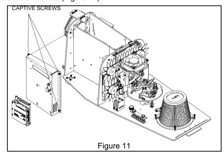
4. Slide the Control Module upwards until it is free from the rest of the PLASI 2000 System.
