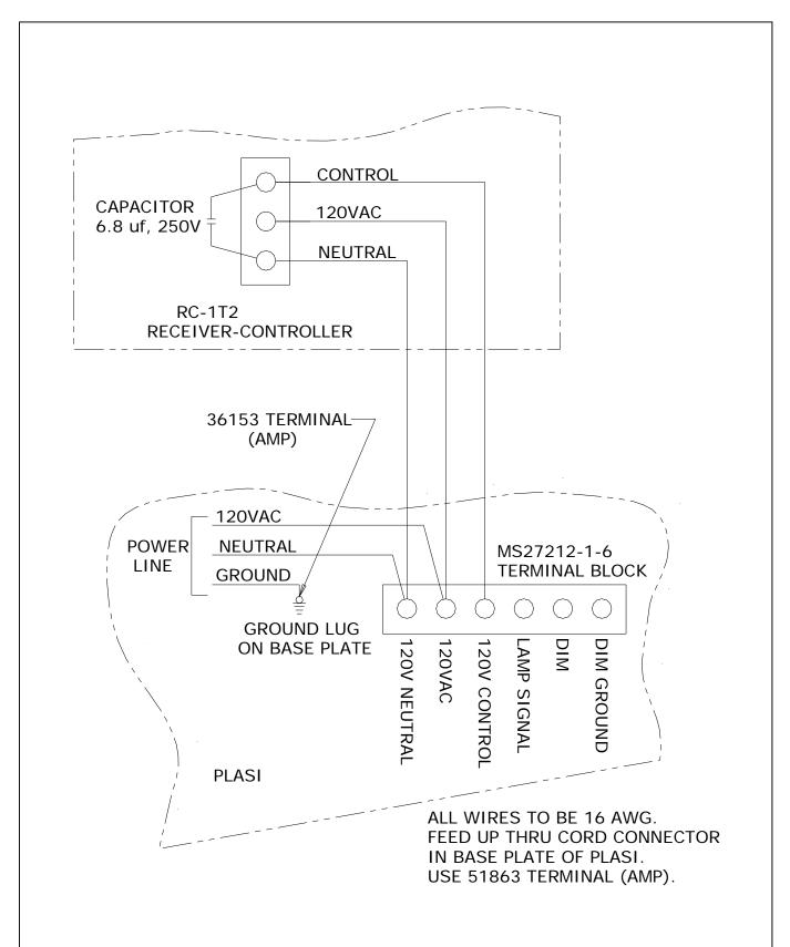
Figure 17 Interconnect Diagram-PLASI to Radio Receiver Controller
