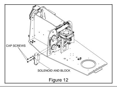
Lens Mount. Retain insulators between Solenoid Block and Lens Assembly, save for reassembly
